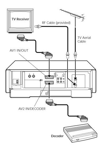
The AV2 IN/DECODER connector can be used as an input terminal for an external decoder (descrambler). Simply connect a decoder and you can enjoy the variety of programming that is available through scrambled channels.
